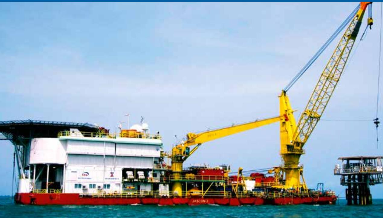
Jascon 2 is an offshore pipe lay / accommodation barge with an 8-point mooring system suitable for pipe lay and other construction work in shallow water environments.
