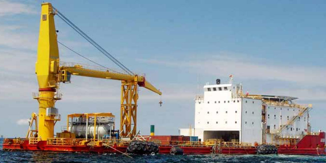
Jascon 8 is a non-propelled anchored offshore barge suitable for accommodation hook-up and commissioning services as well as a great variety of subsea installation and construction activities in shallow water environments.
